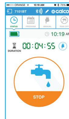
You can stop the irrigation by tapping stop in the status screen or in the manual screen. Manual irrigation does not affect the existing irrigation program. The program will continue as usual, once manual irrigation ends.
